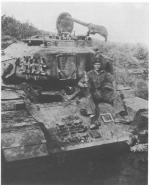
Tpr. Wells, the gunner of 'Black Bob', holds aloft a 3.5-in. bazooka rocket found on the day after the Hook battle in which the tank was pierced by bazooka, wounding the driver. The penetration hole can be seen in the glacis plate just below the driver's hatch beside Tpr. Wells. The hole was repaired by inserting a track pin, cut to length and then welded into position. (Peter Williamson)
