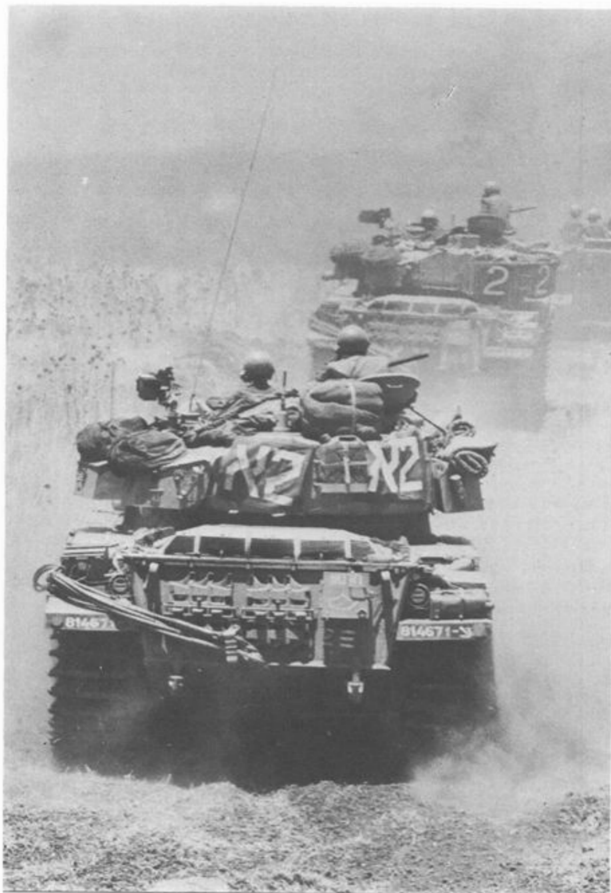
The Centurion will remain in service with the Israeli Armoured Corps for many years to come. These Centurions, during an exercise on the Golan in 1979, are of the latest type with additional armour on the glacis plate, hence the spare tracklinks on the rear hull. Of interest are the loader's machine gun and the new 'Tal cupola'. As an exception to the rule, the nearer Upgraded Centurion has no turret stowage basket. (Israeli Army)
