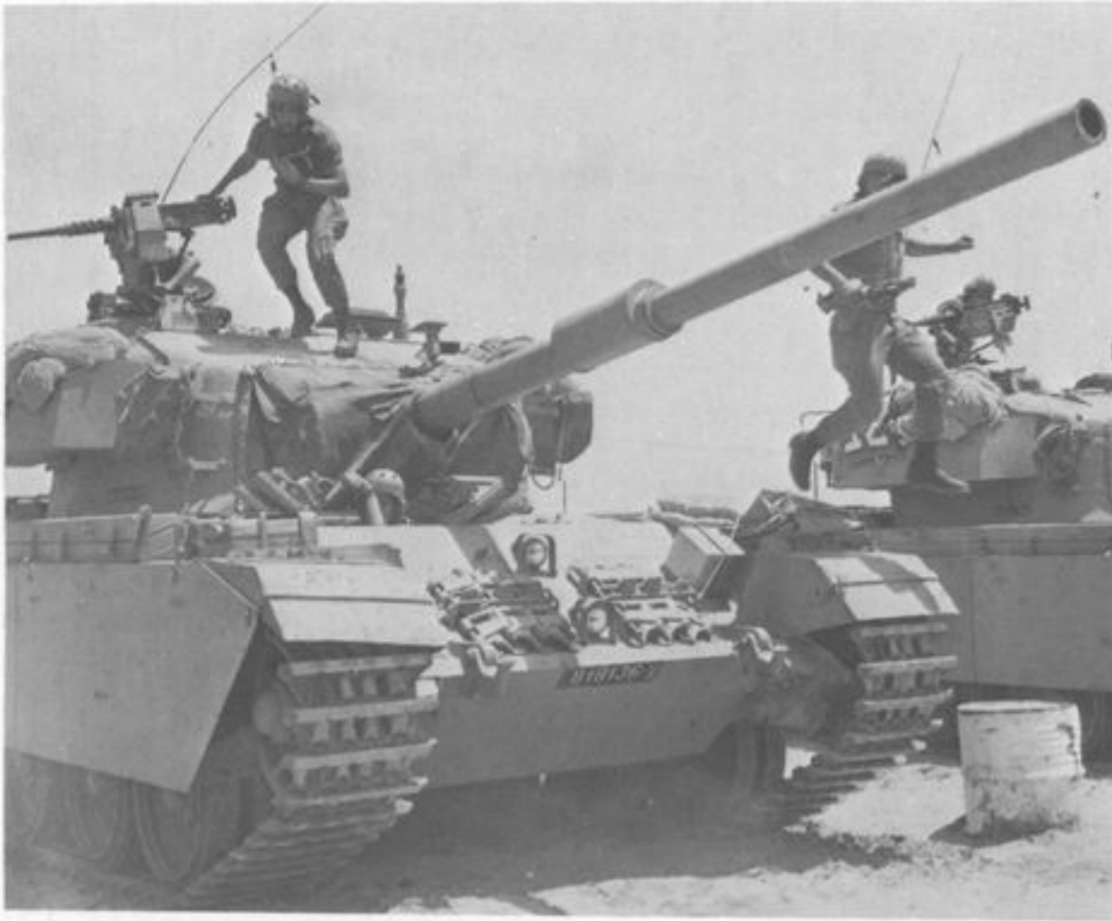
Centurion Mk.5 in the Sinai Desert at the outset of the Six-Day War. Typical of this period, the Centurions have .50 cal. M2HB Brownings at the commanders' cupolas, and the crews wear American tankers crash helmets with Uzi sub-machine guns as personal weapons. (Israeli Army)
