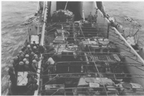
Dawn, 6 November 1956: an LCT carrying elements of 'C' Sqn. 6 RTR approaches the beaches of Port Said at the outset of the assault landings. The Centurions Mk.5 are fitted with metal trunking wading kits. Of particular interest, the leading Centurion tows two one-ton trailers carrying spare 20 pdr. rounds and ammunition as replenishment for the Royal Marine Commandos who landed first. (James Haddon)
