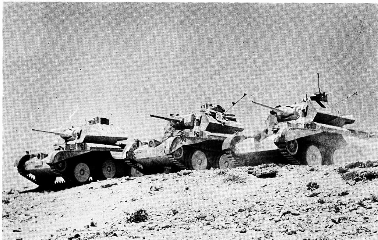
A13 Mk IIs photographed in August 1941. Visible are differing mantlet patterns, a steel helmet used as a headlight cover (right), and a small squadron mark on the turret front (centre)—possibly indicating 2nd Armd.Div., who authorised this practice.
