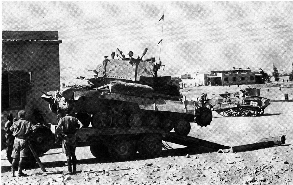
Before the arrival of the Diamond-T Transporter the recovery of untowable 'dead' tanks was more difficult. This A9 is being hauled on to a light trailer for 'back-loading'; the striped bar on the turret may identify a navigator's tank.
