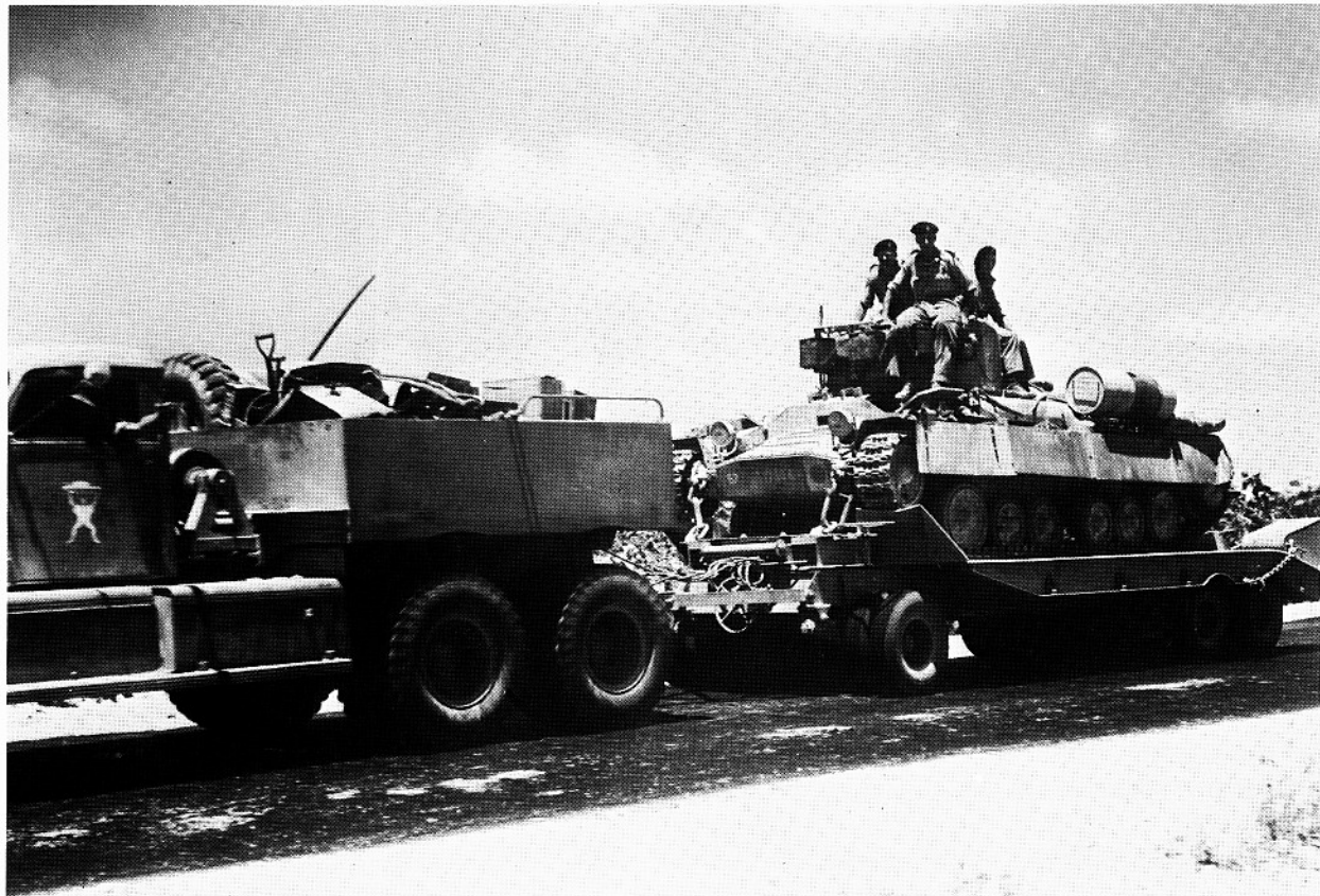
Diamond-T of No. 1 Tank Transporter Coy. RASC lifts a 50 RTR Valentine to the forward area, July 1942. The yellow 'strong man and tank' was the company insignia. Both vehicles are overall Light Stone. Valentine T.17644 carries the number on nose and sides, a large 'C' Sqn. circle, the unit serial '67' and an overpainted 8th Armd.Div. sign.; note jettison fuel tank.
