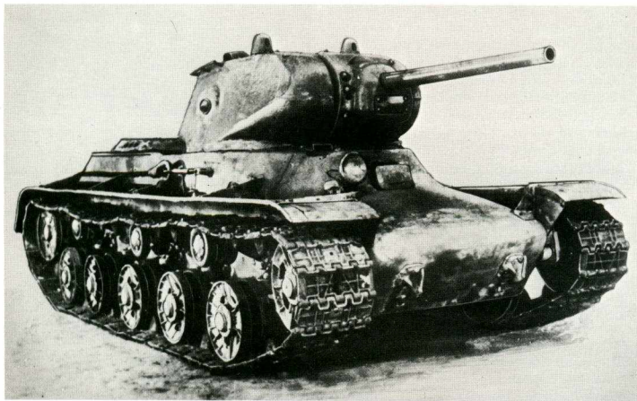
The KV-13T was one of a series of experimental designs which evaluated new heavy tank components; the hull armour layout later used on the IS-1 can be seen on this prototype.
