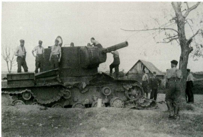
This lone KV-2 Mod. 1940 of the 2nd Tank Div. held off repeated attacks by 6th Panzer Div. near the Rasyeinyia cross-roads in Lithuania. The damage caused by the engineer demolition charges on the right track is evident here. (James Crow)
