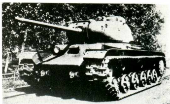
The KV-85, in which the turret of the IS-1 was married with the hull of the KV-1S; note widened superstructure to accommodate larger turret race.
