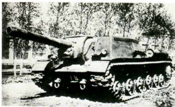
The SU-152 prototype, built in only 25 days in response to the threat of the German Tiger E tank.
