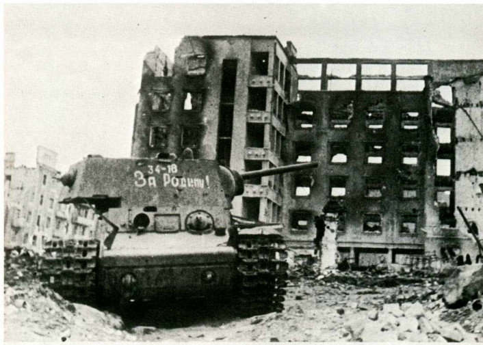
One of the handful of KVs employed in Stalingrad, this Mod.1941 with the newer up-armoured turret is seen supposedly blasting German sniper positions; the turret marking is '34-18' above 'For the Homeland!' (Sovfoto)
