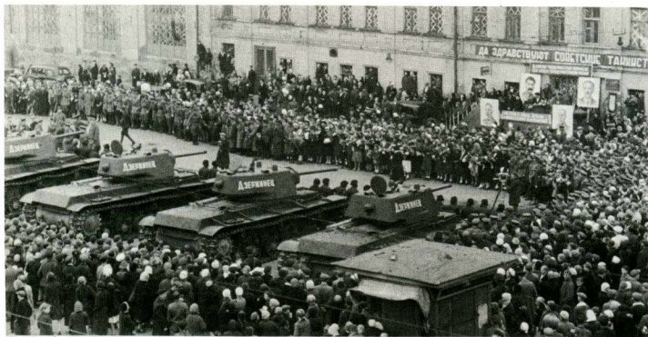
One of the frequent presentation ceremonies, at which local dignitaries would hand over tanks paid for by the contributions of local communities; here, a citizens' group in Moscow hands over a company of KV-1s Mod.1942 to their crews, the turrets inscribed 'Dzerzhynets'. The up-armoured hull of this variant can be identified by the sharp angles of the previously rounded rear engine deck. The turrets are, from left to right: up-armoured cast, standard cast, standard cast, and up-armoured welded. (Sovfoto)
