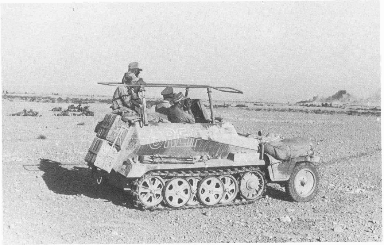
Perhaps the most famous 250 of all – Rommel’s personal command vehicle ‘Greif’ (Griffin) passing through infantry outposts on the fringe of a tank battle in N. Africa, 1942. Note extra racks for jerrycans welded on the rear hull. (Bundesarchiv)
