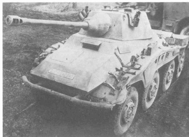
Abandoned SdKfz 234/2 Puma heavy armoured car fitted with a primitive but robust barrier shield. The smoke grenade dischargers, set to throw a pattern of bombs across the front of the vehicle, were an invaluable aid when reversing out of trouble. The colour scheme is ochre, possibly with a faint overspray of green or brown blotches, but so weathered and dusty as to be almost monotone. (RAC Tank Museum)
