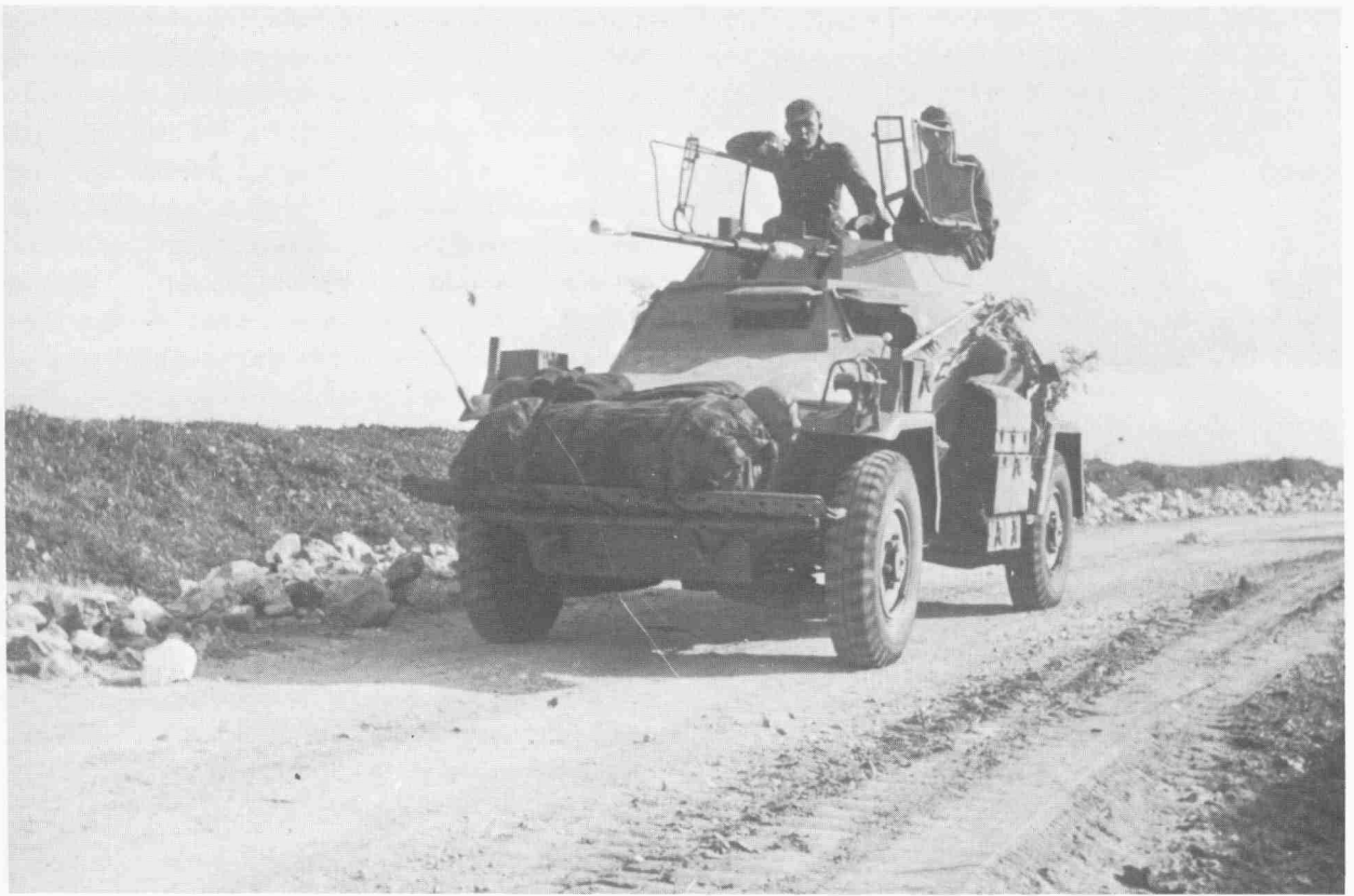
SdKfz 222 in Tunisia, 1943; after two years of desert warfare neat, workmanlike stowage has become a matter of routine. A few fronds of greenery have been added to the vehicle's camouflage, as the Tunisian spring has changed the overall aspect of the landscape. (Bundesarchiv)
