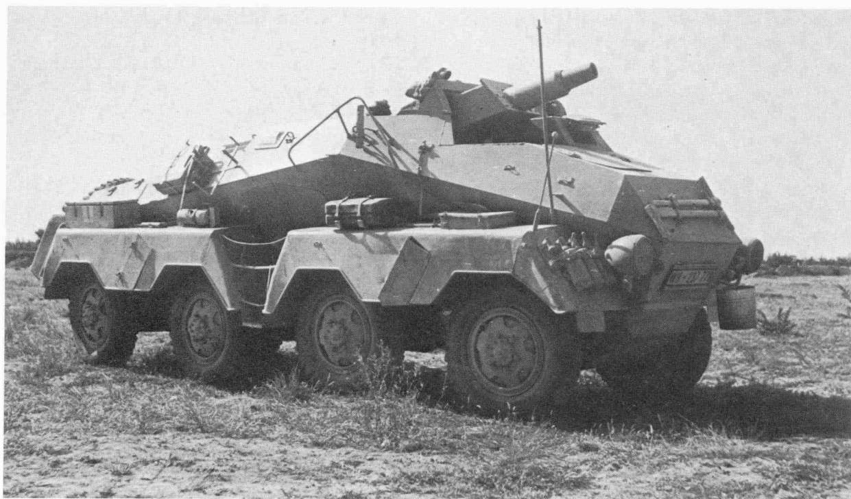
Nice study of an SdKfz 233 (8-rad) 75mm captured in N. Africa in almost new condition. The only marking on the neat sand-coloured overspray is the numberplate. (RAC Tank Museum)
