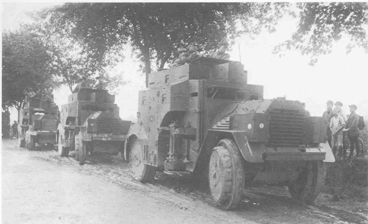
Daimler Gepanzerter Mannschaftstransportwagen (SdKfz 3) of the Reichswehr on manoeuvres in East Prussia in 1928. These MTWs were unarmed armoured personnel carriers; under the Allied Control Commission regulations only the Schutzpolizei were permitted true armoured cars. (Bundesarchiv)
