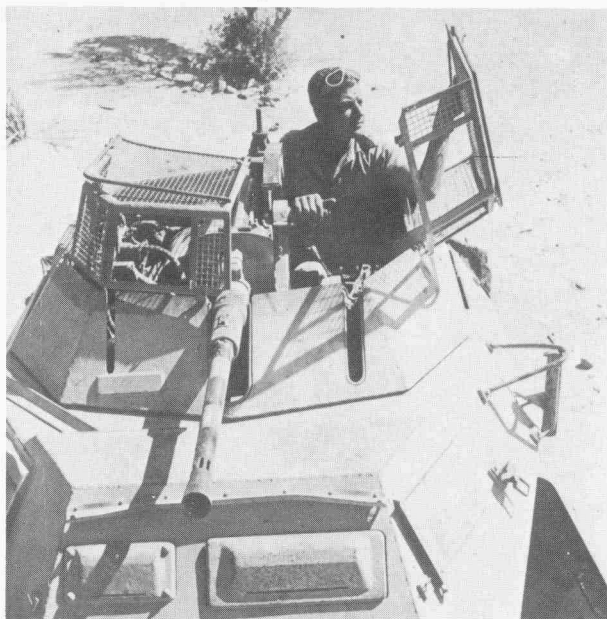
Detail of the 20mm mounting and anti-grenade grilles of an SdKfz 222 – the co-axial MG is absent. (RAC Tank Museum)
