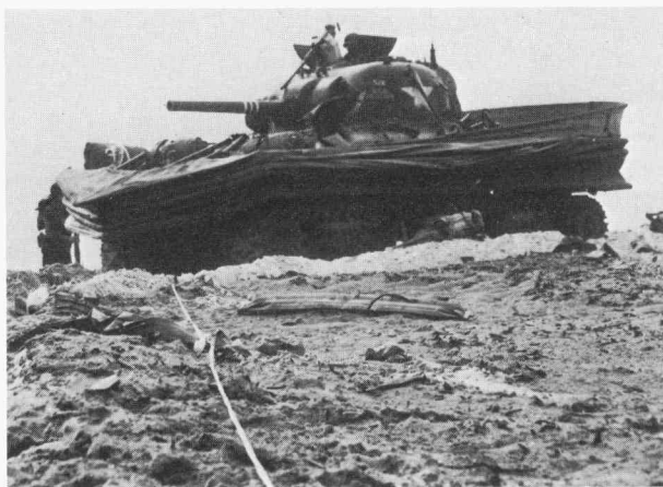
An M4A1 Duplex Drive (DD) Sherman of the 756th Tank Bn. supporting troops of the 15th Inf. Regt. at Alpha Yellow Beach (Pampelonne) on 15 August 1944 during the invasion of southern France. The DD tank was a regular Sherman with an erectable flotation device designed to enable it to swim ashore from landing craft. They were used with mixed results during the Normandy landings by three US tank battalions, and were also used by American forces during the Rhine crossings.
