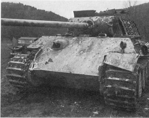
A close-up look at a PzKpfw V Ausf. G Panther hit by eight rounds of 76mm APC near Saverne, France. The gouges of six of these rounds are evident, only the hit on the lower left corner of the glacis plate causing a minor penetration. The 76mm gun could only get penetrations against the front of the Panther by using the scarce HVAP ammunition, or by firing from a dangerously close range.
