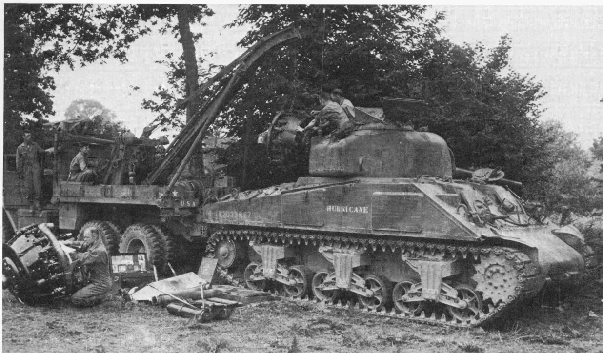
'Hurricane', an M4 of 'H' Co., 66th Armd. Regt., 2nd Armd. Div., has its Whirlwind engine removed with the aid of an M1 Wrecker. Like most of the tanks of 2nd Armd. Div., this M4 was camouflage-painted shortly after landing in Normandy with a pattern of Earth Brown over the usual Olive Drab. This repair work was being done near Le Teilleul, France, on 17 August 1944.
