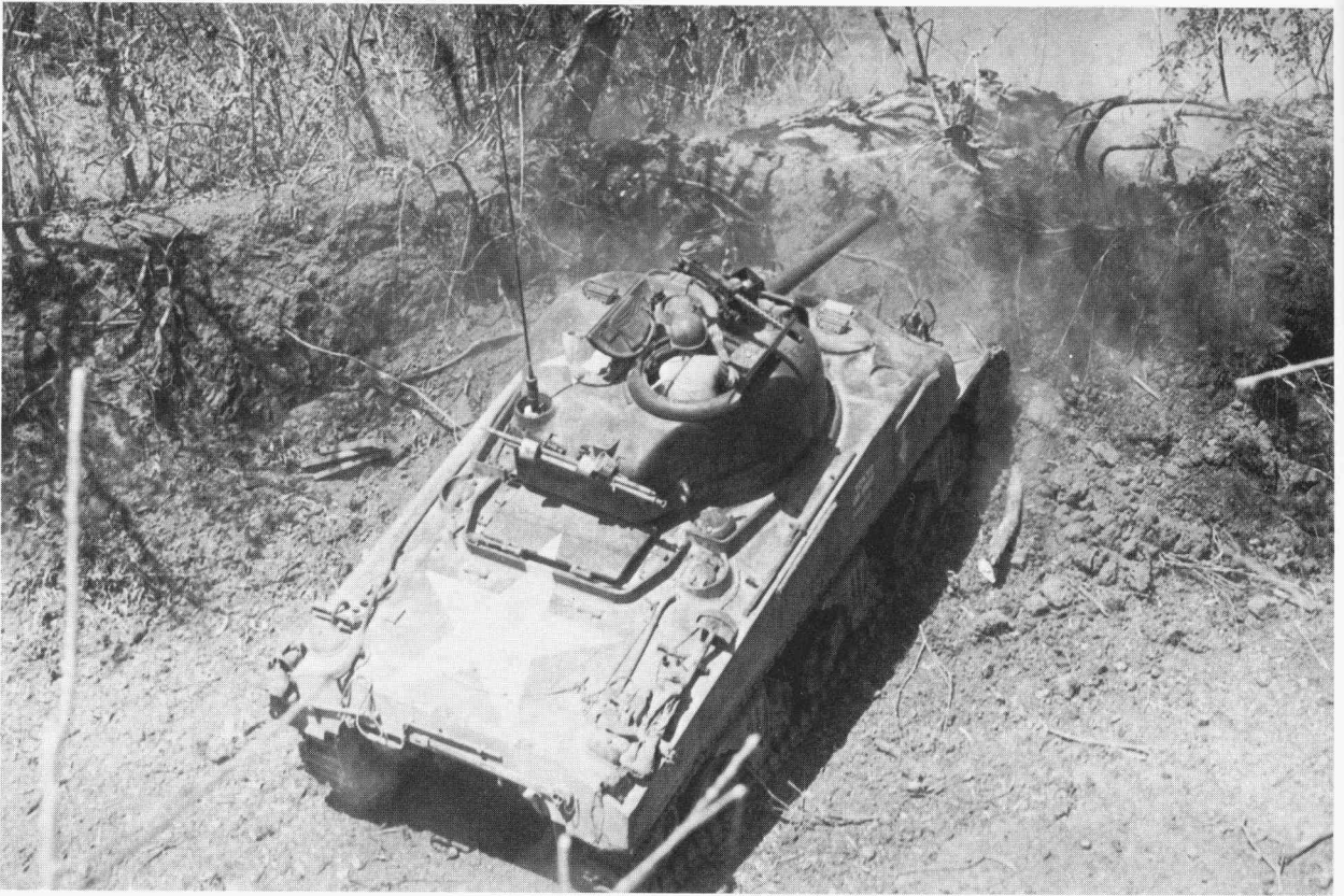
A late production composite-hull M4 of the 44th Tank Bn. fires into a Japanese gun pit in the outskirts of Manila during the Philippines fighting, 10 March 1945. The composite-hull M4 had a cast front end and a conventional welded rear hull superstructure. This view shows the large air identification stars to good effect.
