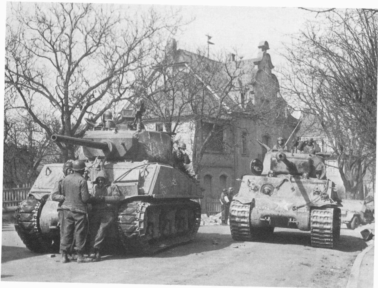
An M4A3E2 'Jumbo' (left) and M4A3E8 of the 37th Tank Bn., 4th Armd. Div. pass through Alzey, Germany, on 20 March 1945. The Sherman on the right is an HQ tank and is either Maj. Bautz's tank, 'Tornado', or Col. Creighton Abram's 'Thunderbolt'. (One of the earlier 'Thunderbolts' is shown in Plate Br.) The thick turret frontal armour on the Jumbo is very evident in this view. This particular assault tank has been re-armed with a 76mm gun; initially the Jumbos were armed with 75mm guns.
