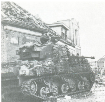
A well-armoured Sherman Firefly of 10th Armd. Cavalry Bde. during the fighting for Moerdijk, November 1944. Note the addition of ammunition boxes to the rear of the turret bustle.
