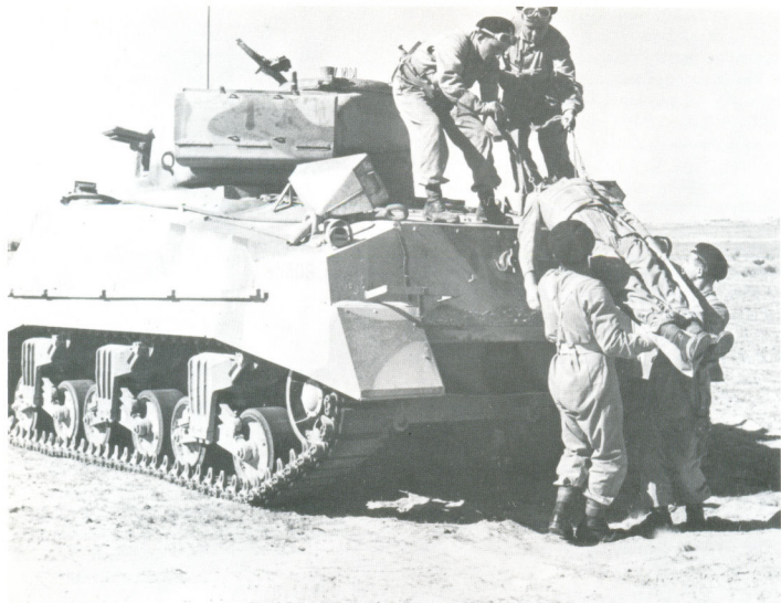
A scene during exercises by 2nd Armd. Bde. in Egypt, shortly before it was to join the fighting in Italy. The Sherman is probably in desert finish of Light Mud and Blue-Black. Note the large funnel on the rear of the vehicle.
