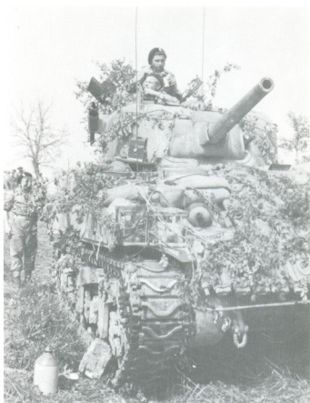
Sherman of 2 Sqn., 4th Arm'd. Regt. 'Skorpion' commanded by Officer Cadet Jarzembowski, shortly before moving into action at Monte Cassino, May 1944. Note the additional protective layer of sandbags. In the original print the black scorpion emblem is just visible on the turret side, partly obscured by the periscope and branches of the camouflage.
