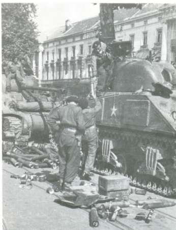
Men of the 24th Lancers re-ammunitioning their 'chargers' at Ghent, Belgium, September 1944. Note the typical appliqué plates welded onto the hull sides, as well as the considerable number of slogans and messages chalked on the hull.
