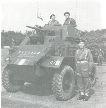
Humber armoured car of Maj. Zbigniew Dudzinski, commanding officer of 1st Reconnaissance Regt., 1st Armd. Div. at Dalkeith, Scotland, on 29 May 1943. The markings carried include the formation sign, unit code (white '47' on black), red/white/red AFV recognition sign and the tactical sign. Note the Regimental Guidon, topped with the 1st Armd. Div. insignia.
