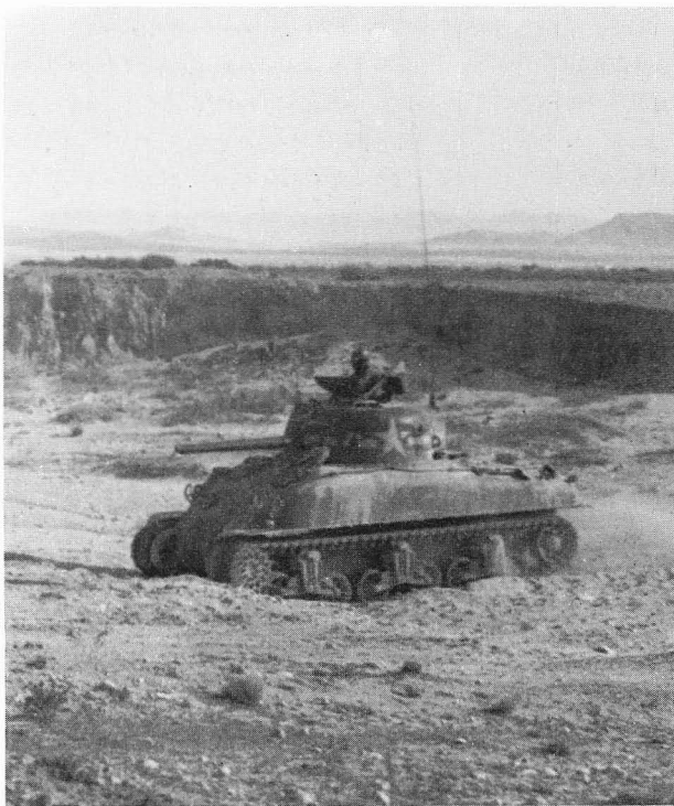
An M4A1 Medium Tank of 2nd Platoon, Co. G, 3rd Bn., 1st Armd. Regt., 1st Armd. Div. crossing a river bed at Sidi Bou Zid on 14 February 1943. The markings consist of the divisional tactical insignia on the turret front; the national insignia with the tank number '3' in the centre; and two dots indicating 2nd Platoon behind the pistol port on the turret.
