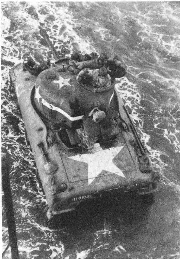
An M4A1 Medium Tank of the 710th Tank Battalion off the San Clemente, CA coast on 16 February 1944. This view shows the full range of national markings outlined in the AR-850-5 and technical bulletins, including the prominent turret band. The bumper codes 'III-710 Δ', 'HQ13' indicate 13th vehicle of the HQ Co., 710th Tank Battalion, III Corps.
