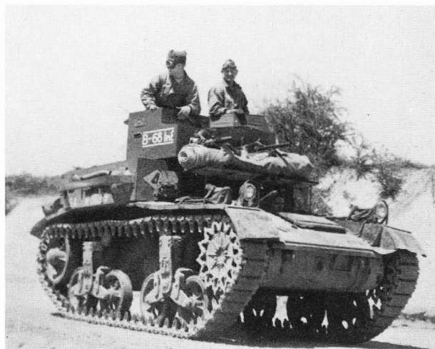
A 'Mae West' (M2A2 Light Tank) of the 3rd Platoon, Co. B, 1st Tank Battalion, 68th Infantry (Light Tanks) at Ft. Benning in April 1940. This tank displays markings fairly typical of the inter-war period. The turret unit designator is an authorised, alternate style to the type seen on the photo here of the T3 Christie tank of the 67th Infantry. The red diamond with black '4' seems to be related in style to the markings adopted by 66th Infantry.
