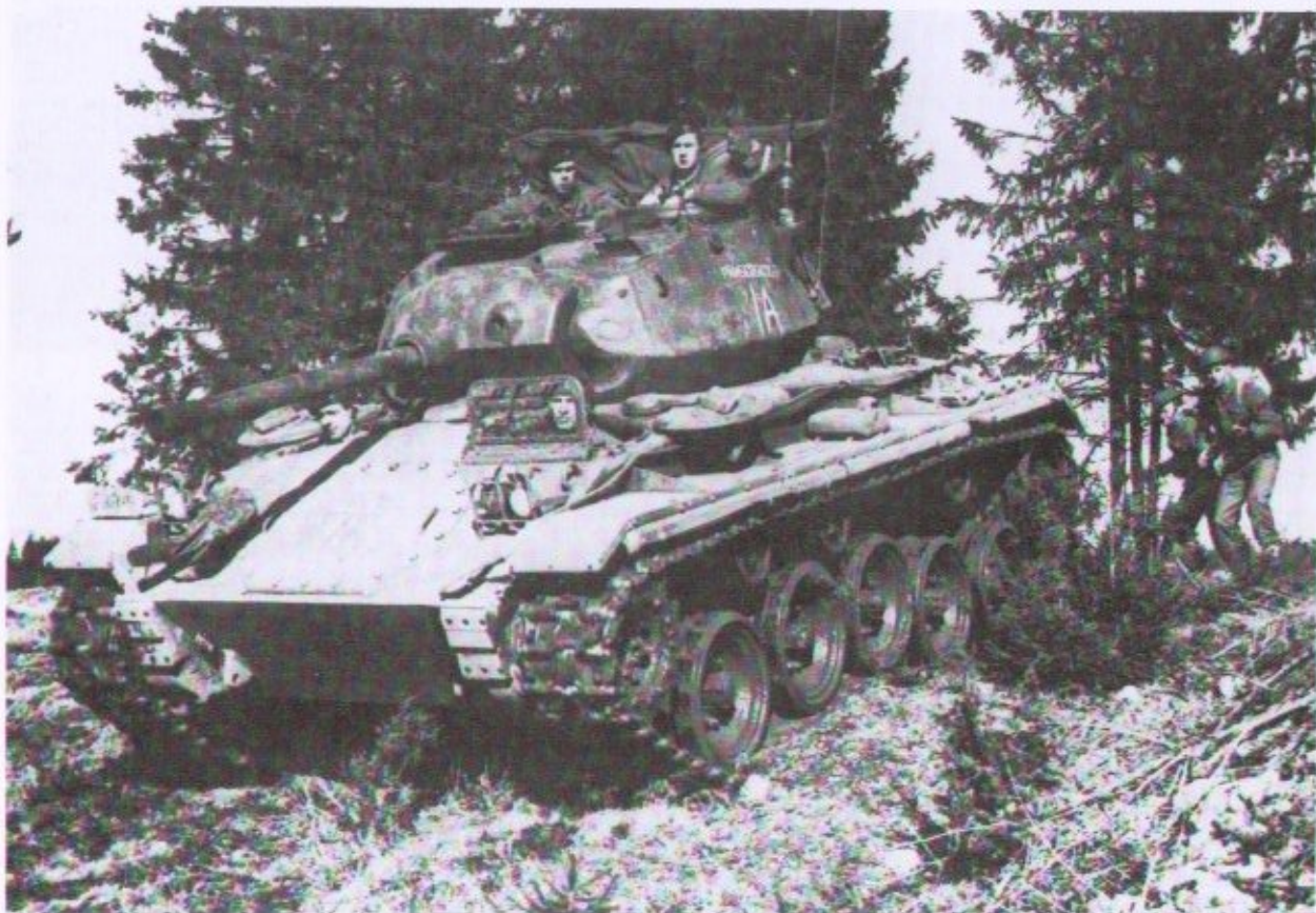
A Chaffee of the Norwegian Panserkolen on exercise in the 1950s. These tanks were rebuilt in the 1970s, and are still in service! (National Archives)
