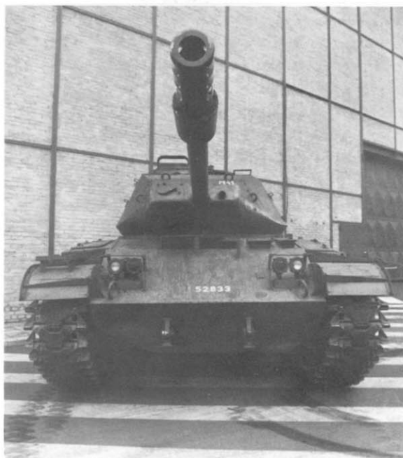
The Belgian firm of Cockerill proposed to extend the life of the M41 by substituting this improved Mk IV 90mm low-pressure gun for the original 76mm weapon. (Cockerill)
