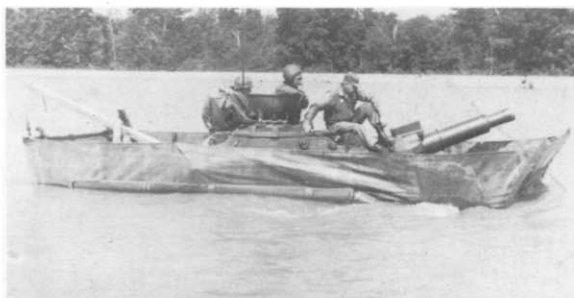
As befitted a scout vehicle, the M551 was designed to be amphibious. A screen was contained in hull recesses, and could be erected before entering the water; propulsion was by means of the tracks. This early production vehicle, photographed on trials, is still fitted with the bore evacuator and open-breech scavenger system. (US Army)
