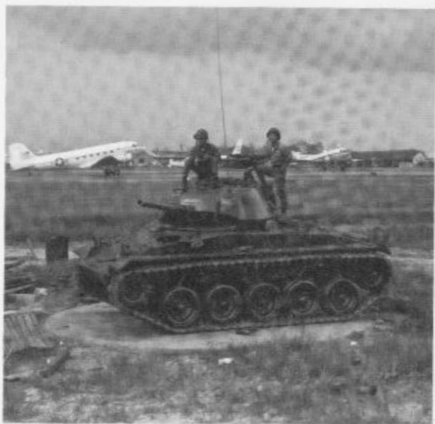
When replaced in South Vietnamese armoured units by M41s, many M24s had their engines removed and were turned into static pillboxes. Some were retained by the South Vietnamese Air Force as anti-coup security for Premier Ky, and were used to patrol the perimeter of Tan Son Nhut Airbase. See Plate C1. (US Army)
