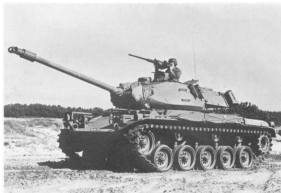
This Danish Army tank is an M41A1, but it is almost impossible to distinguish sub-types of this series from photos—all major differences were internal. (Danish Army)
