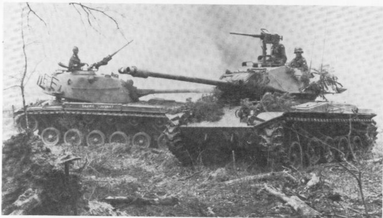
An M41 Walker Bulldog of the 2nd Armored Cavalry Regiment exercises at Ft. Meade, Maryland, with an M48 Patton: April 1957. (US Army)
