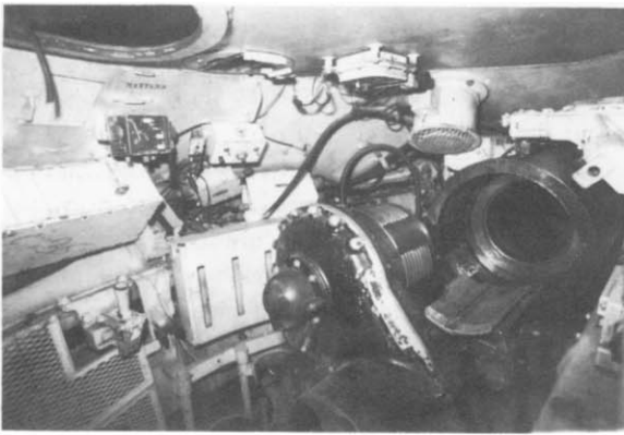
Interior of the M551 turret, looking from the commander's station forward and left towards the loader's station. The unconventional breech design is very evident in this view. (Zaloga)
