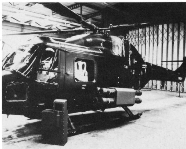
Increasing attention is being paid to the use of attack helicopters to fight hostile attack helicopters. This shows a test fitting of the Swedish Bofors RBS-70 anti-aircraft missile, mounted on a modified Westland Lynx helicopter. (Bofors)
