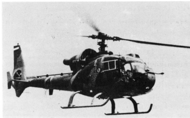
An Iraqi SA.342M during the 1984 fighting with Iran. This helicopter is fitted to carry the HOT missile, which is not loaded in this view.
