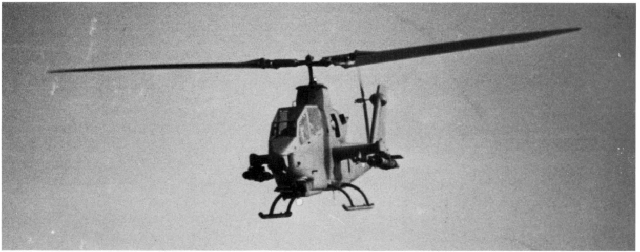
An Israeli AH-1S armed with four TOW missiles. This view underlines the small target that an anti-tank helicopter presents during 'pop-up' attack. (Government Press Agency)
