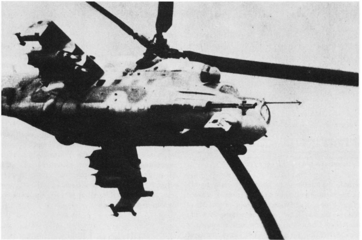
An Mi-24 'Hind-E' of the later type with the twin 23mm autocannon on the starboard fuselage side and launch mountings for the AT-6 'Spiral' anti-tank missile. This helicopter was taking part in the 1985 Kavkaz-85 exercise. Note that this version lacks the nose gun barbette, like the training version of the 'Hind-D'.
