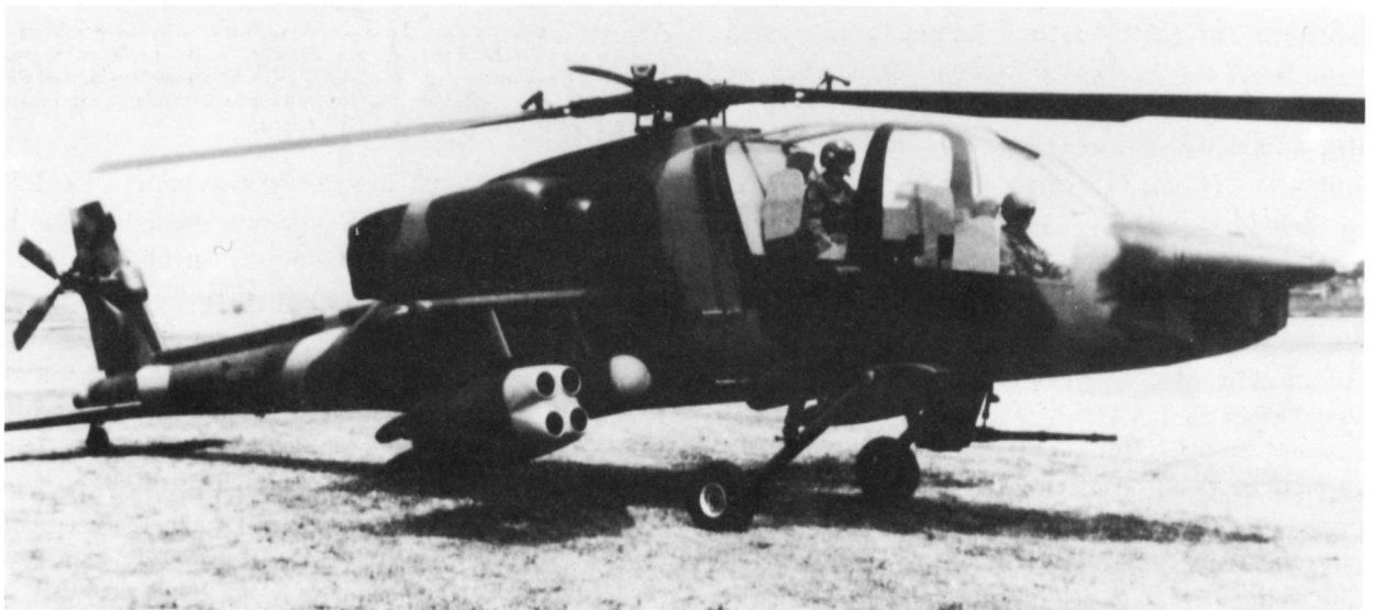
This photo shows the original conception of the Hughes YAH-64 prototype, which eventually evolved into the AH-64 Apache. (US Army)
