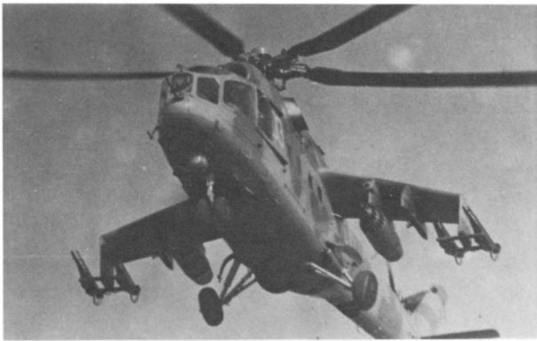
The Mi-24 'Hind-A' was originally powered by the Isotov TV2-117 engine, and had the tail rotor on the starboard side of the tail. This view shows one of these early 'Hind-As', armed with two UB-32 rocket pods and launch racks for the Falanga guided anti-tank missile. (US Navy)
