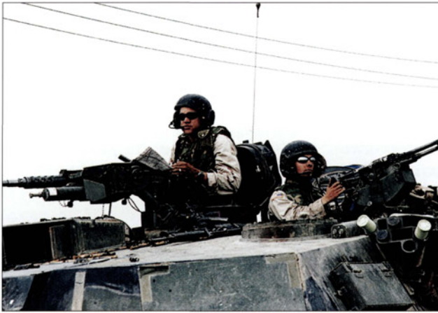
The tank commander (left) and loader man with their respective .50-cal. and 7.62mm machine guns on an M1A1 tank. None of the tanks of the 1st Armored Division changed out of their European camouflage paint scheme for this campaign. The men wear Interceptor vests and commercial ballistic eyewear. Their M4 carbines remain ready to use, the commander studies his map; the spent cartridge cases indicate he has used his machine gun recently.
